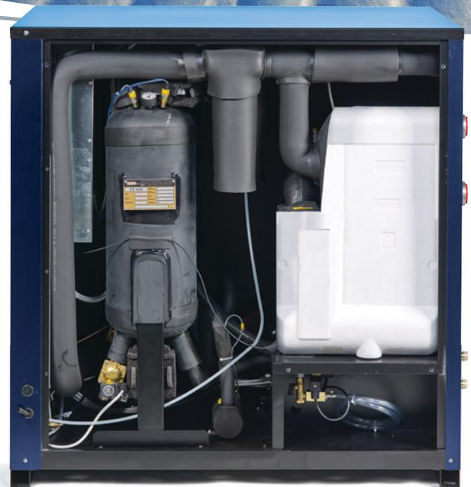
Technology exploiting both PSA (pressure swing adsorption) and TSA (temperature swing adsorption) brings together an effective and economical solution to meet the needs of the compressed air user. With the addition of a dew point dependent switching feature for periods of intermittent load, incorporated into the electronic controller of every CDT dryer, initial investment costs are quickly amortised and life-time costs minimised.
